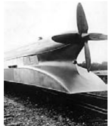
German inventor Franz Kruckenberg designed the track zepplin in 1930. The car resembled an airship, ran on tracks like a train, and used propellers to achieve speeds of more than 100 mph.
